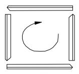
The final piece needs to have its square cut end tucked under the first piece's coped end prior to snapping in place.
